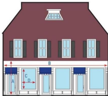
A: Height of Ground Floor B: Width of Ground Floor C: Height of Glazing D: Width of Glazing
